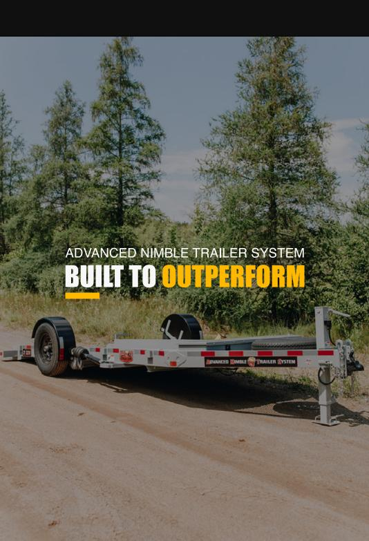
A versatile and reliable hauling solution for your transportation needs. With a load angle of 3 degrees on the bed and 9 degrees on the ramp, this trailer ensures easy and efficient loading and unloading of your cargo.
